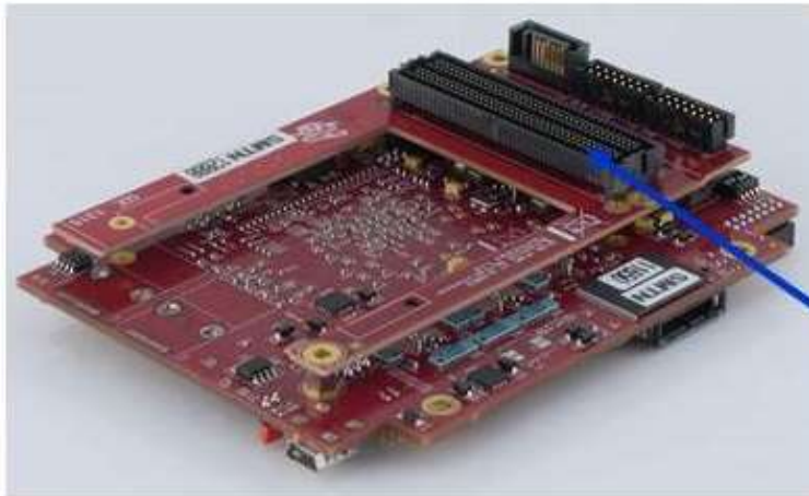
Figure 5 SMT105 PCIe/104 FPGAs Module gets more I/O options with VITA57.1 FMC Add-on Module
