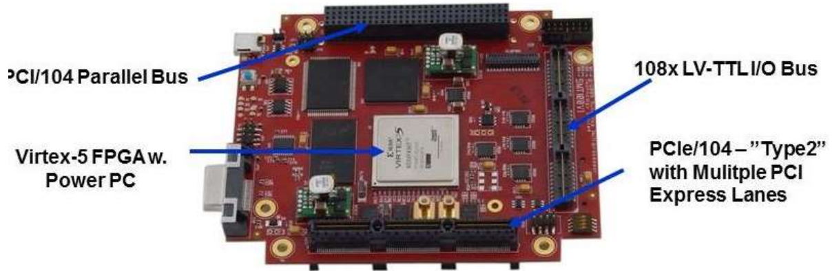
Figure 3 Dual Core PowerPC integrated into a Virtex-5 FPGA on a PCIe/104 Module
