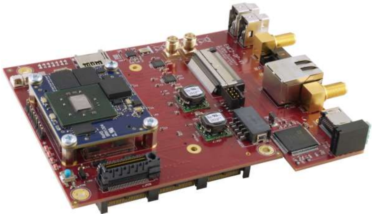
Figure 2 The EMC 2 showing the Stackable PCIe/104 OneBank Connector and the Cable-less I/O board
