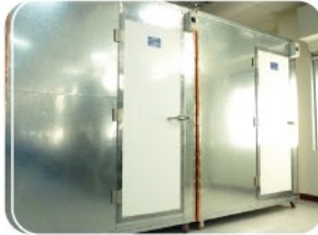
The Shielded Room is designed to prevent waves leak-in. ▶
