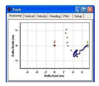
When Navigation Speed Threshold is enabled, notice that there is a significant reduction in drifting. The drifting for East/West direction is now limited to 2 meters, and 6 meters for the North/South direction.
